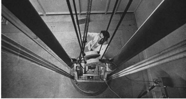
"THE GUILLOTINE" is the nickname of this new drop machine undergoing evaluation by Stan Kurowski. The machine is expected to give a 400 lb. test unit shocks up to 2000 g's in two milliseconds. Carriage can reach a velocity of 70 miles per hour at the moment of impact.
